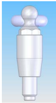
Fig 2: Drawing of O ring attachment showing O ring in ideal position below rounded ball
